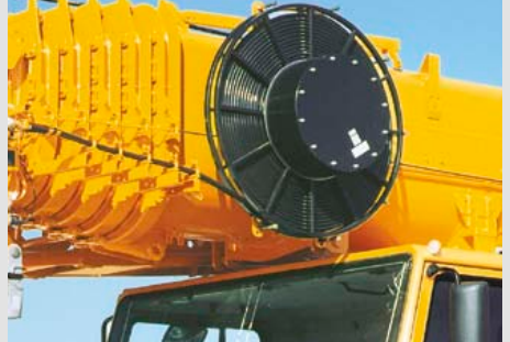
Hose drum for hydraulic cylinder
