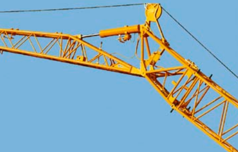
Hydraulically adjustable swing away jib (0° - 40°)
